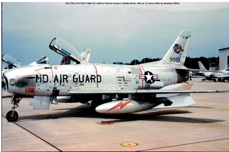
One of the MDANG's F-86H Sabres at Martin Airport. The soot on the nose means that the 20mm cannons were recently fired. (Image from 1963 by Stephen Miller from the internet.)
